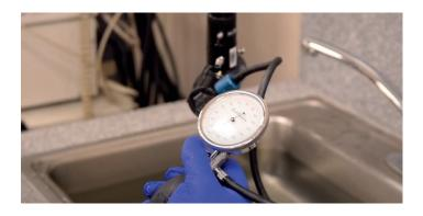
The second and preferred method is to use a hand-held pressure tester. The benefit associated with using a hand-held is that it allows the user to see if there is a leak in the scope **before it is submerged in the water**. The user pumps air through the scope, via the ETO valve, to hold a determined amount of pressure.
