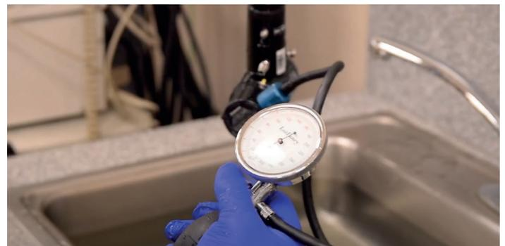
The second and preferred method is to use a hand-held pressure tester. The benefit associated with using a hand-held is that it allows the user to see if there is a leak in the scope **before it is submerged in the water**. The user pumps air through the scope, via the ETO valve, to hold a determined amount of pressure.
